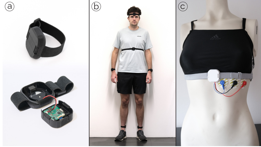
Figure 1: Our sensing platform enables the use of multiple sensing devices simultaneously. The custom electronics of each device are integrated into a 3D-printed enclosure along with the battery (a). Thanks to adjustable straps of various lengths, the devices can be placed in any body location. The proposed on-body placements include the wrists, ankles, forehead, and sternum (b). The device can be connected to gel-electrodes to record reliable Lead I ECG (c).
