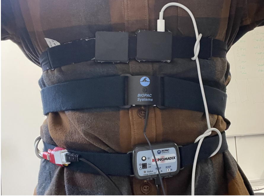
Figure 26: The device setup on the participant’s thorax for the study included the custom UWB device which was strapped over the sternum, followed by the reference respiratory belt over the abdomen, and the transmitter of the respiratory belt.
